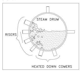
The boiler was provided with heated down comers. There were no baffles inside the drum to separate the steam water mixture from down comer section. When the load in the boiler increased beyond a point the down comers started bursting.
