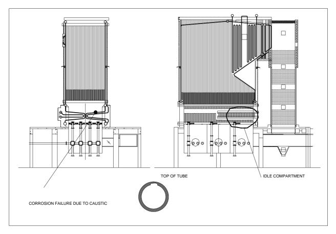
The above is a Fluidized bed combustion boiler with three compartments. A pin hole failure was reported in the 12 o clock position of the bed coil tube. On cutting the tubes, the inside was found have gouging mark for the throughout the inclined portion of the tube. Several adjacent tubes are inspected with D meter. Four adjacent tubes showed less thickness at 12o-clock position. The tubes were cut inspected and these tubes were also found to have the same marks as the leaked tube.
