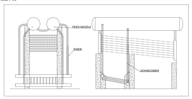
This boiler was converted for fluidized bed firing. There were wrinkle formations in bed coil tubes. It was felt that the Downcomer & risers were inadequate and several modifications were done in order to reduce the pressure drop in the circuit. Still the failures continued. Suspecting boiler expansion problem, the refractory work was reconstructed with adequate provision for expansion. Yet the failures continued.
