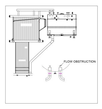
In this case, the water wall & bed coils were failing after bulging & overheating. Thick rough edge cracks were observed wherever the failure took place. There were several locations at which the failures had taken place.
